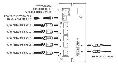
Figure 6. FX82051 Module Connections
